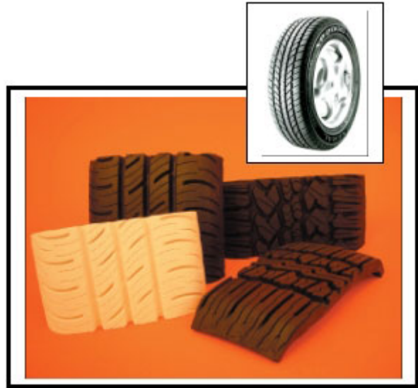
The Continental ContiProContact was recently introduced by Continental Tire North America in 22 sizes with advancements in wet traction and handling. The ZPrinter 310 provided the engineers with a hands-on evaluation of the tread design before investing in the expense of molds and tire building.
